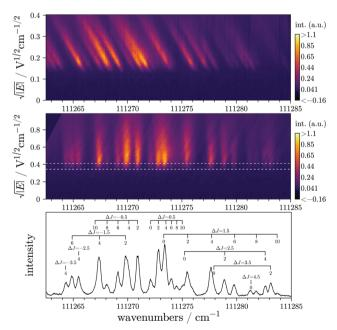
Fig. 6 Experimental measurement of the  $X^{+2}\Pi_{g,1/2}(v^+=0) \leftarrow X^1\Sigma_g^+(v=0)$ transition of CO2 recorded with the PRFI-ZEKE method. The linearized matrix, the rotated matrix, and the final spectrum are depicted in the upper, middle, and lower panels respectively. The color scales are arbitrary. The final spectrum has been obtained by integrating the rotated matrix over the y range delimited by the white dotted lines.
