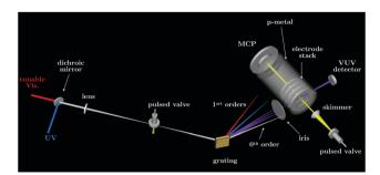
Fig. 1 Sketch of the VULCAIM experimental setup.
