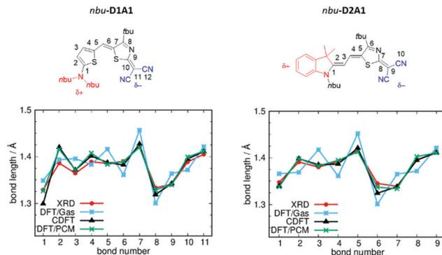
**Fig. 2** Chemical structures and BLA paths (as defined by bond numbering) for *nbu-D1A1* (left) and *nbu-D2A1* (right) merocyanine – upper panels (*nbu-D1A1*, known also as **HB238**).<sup>5</sup> Bond lengths (Å) from XRD data (red lines), DFT ( $\omega$ B97X-D3/6-311G\*\*, gas phase, blue lines), C-DFT (CAM-B3LYP-D3/6-311G\*\*, gas phase, black lines,  $\delta^{D/A} = \pm 0.6q$ ) and DFT ( $\omega$ B97X-D3/6-311G\*\*/PCM(DMSO), green lines) calculations – bottom panels.
