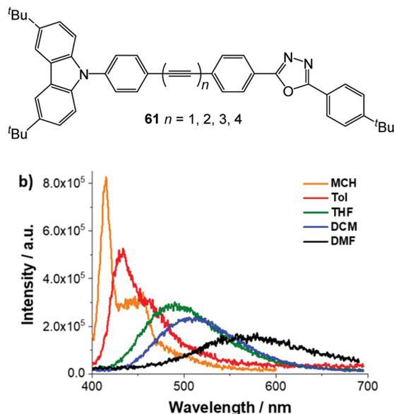
Fig. 20 Structure of **61**. Fluorescence spectra of **61**  $n = 3$  in solvents of different polarity (MCH, methylcyclohexane; Tol, toluene; THF, tetrahydrofuran; DCM, dichloromethane; DMF, *N,N*-dimethylformamide) with matching absorption of OD = 0.05 upon 350 nm excitation. Reproduced from ref. 166 with permission from the American Chemical Society.
