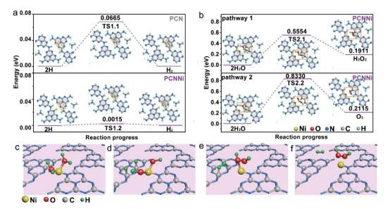
Fig. 6 Reaction pathways of (a) water reduction to  $H_2$  and (b) water oxidation to  $H_2O_2$  (top) and  $O_2$  (down) for PCNNi (single-atom Ni coordinated with sp<sup>2</sup> NA atoms). (c–f) Proposed mechanisms of photocatalytic pure water splitting into  $H_2$  and  $H_2O_2$  for PCNNi (single-atom Ni coordinated with sp<sup>2</sup> NA atoms).
