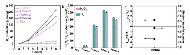
Fig. 4 (a) Photocatalytic hydrogen generation from pure water under visible light ( $\lambda$  > 420 nm), (b) photocatalytic overall water splitting into hydrogen and hydrogen peroxide without any sacrificial reagent under visible light ( $\lambda > 420$  nm) with activity marked by the error bar, (c) the measured Pt disk current and Pt exchange current and corresponding electron transfer number.
