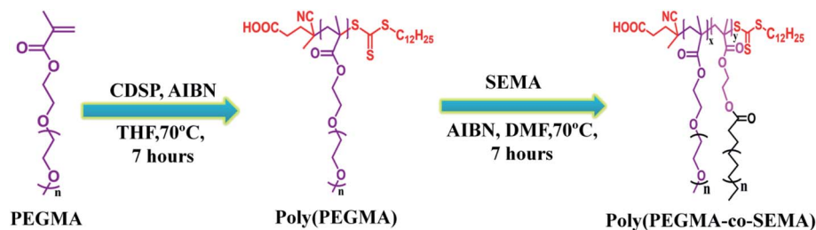
Fig. 1 Synthesis route of PEGMA-co-SEMA block co-polymer.
