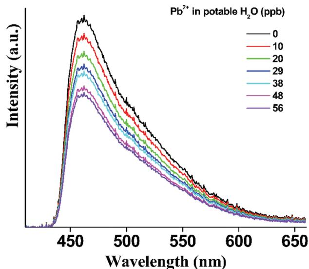
**Fig. 9** The fluorescence titration ( $\lambda_{\text{exc}} = 380$  nm) of a stirred suspension of **p-UCR-20** in water ( $0.1 \text{ mg mL}^{-1}$ ) upon the addition of aliquots from a  $\text{Pb}^{2+}$  standard stock solution (concentration = 1000 ppb) in potable water.
