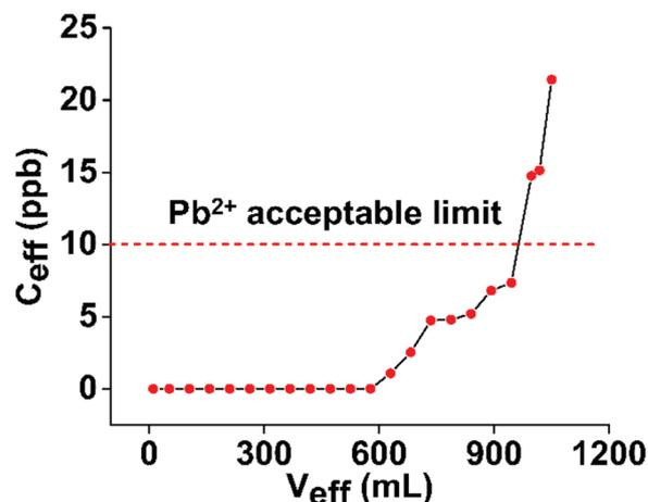
**Fig. 7** Column sorption data with a wastewater simulant solution (flow rate  $\sim 1.0$  mL  $min^{-1}$ , one bed volume = 3.5 mL, stationary phase **p-UCR-20-CA**/sand = 0.05 g : 5 g, initial Pb concentration = 100 ppb).  $V_{eff}$  and  $C_{eff}$  represent the volume (mL) and  $Pb^{2+}$  concentration (ppb) of the solution passed through the column (*i.e.* effluent) respectively.
