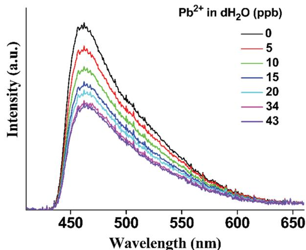
**Fig. 8** The fluorescence titration ( $\lambda_{\text{exc}} = 380$  nm) of a stirred suspension of **p-UCR-20** in water ( $0.1 \text{ mg mL}^{-1}$ ) upon the addition of aliquots from a  $\text{Pb}^{2+}$  standard stock solution (concentration = 1000 ppb) in distilled water.
