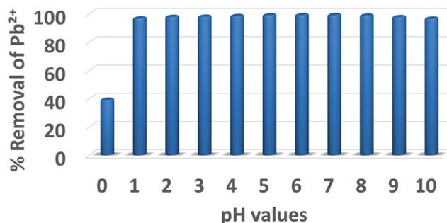
Fig. 6 % Pb<sup>2+</sup> removal by **p-UCR-20** vs. pH.
