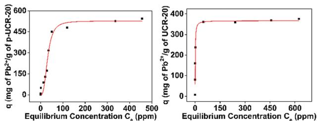
Fig. 5 Isotherm data for Pb<sup>2+</sup> sorption by **p-UCR-20** and by **UCR-20**. The red lines represent the fitting of the data with the Langmuir–Freundlich model. Detailed fitting data are presented in Table S1.†
