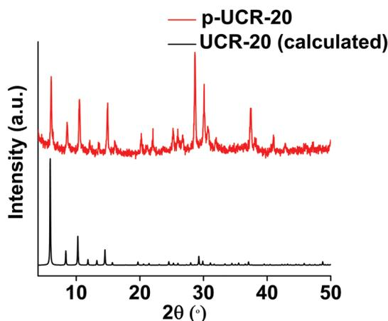
Fig. 2 PXRD patterns of UCR-20 (calculated) and p-UCR-20.
