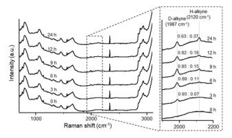
Fig. 4 Average Raman spectra of the lipid region (20 × 20 pixels) of ten HeLa cells treated with 100 μM D-3. Raman spectra after various incubation times (0-24 h). The Raman peak area ratios between D-alkyne and H-alkyne signals at each treatment time are shown.
