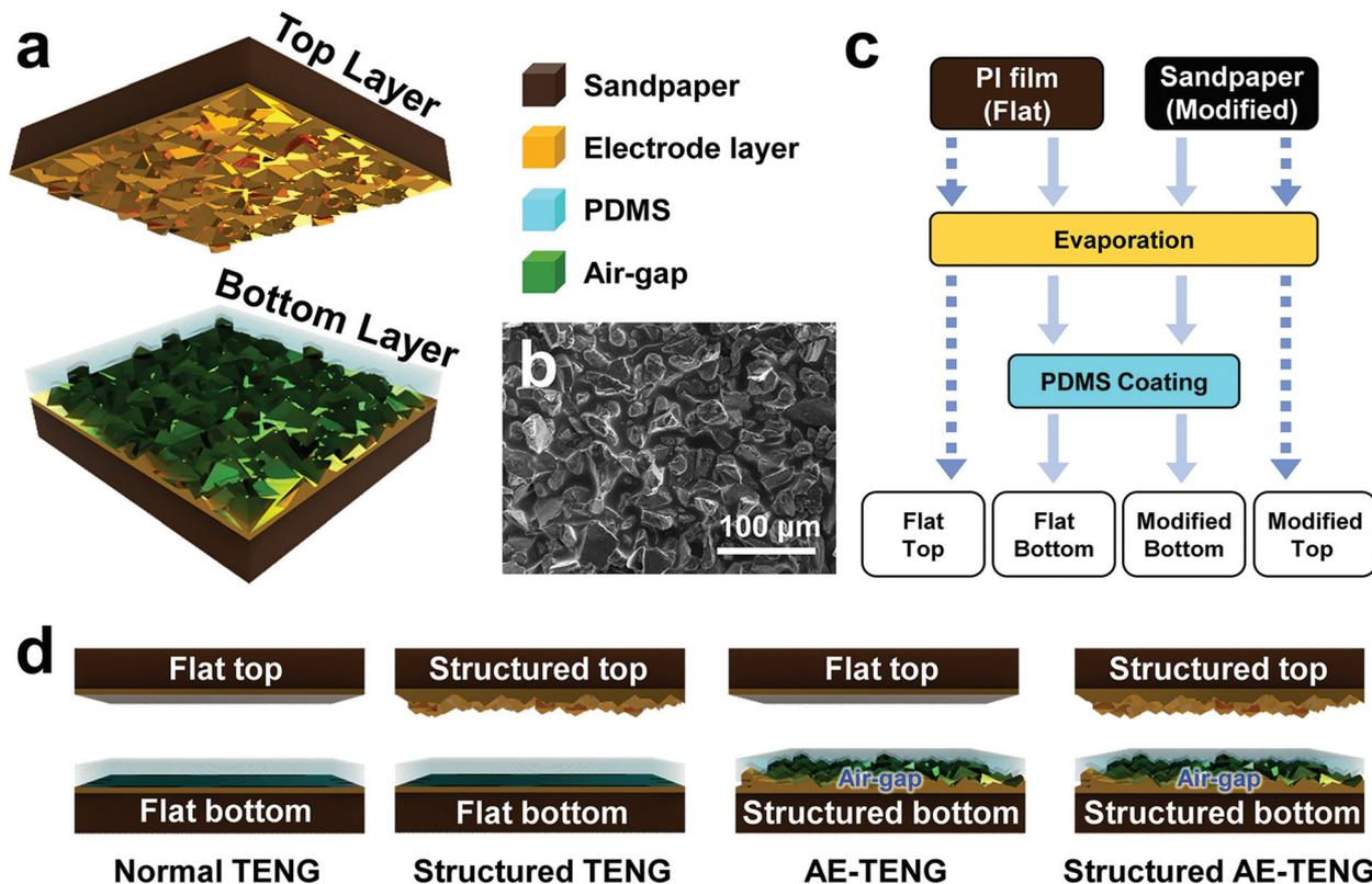
**Fig. 1** (a) Schematic illustration of the structured air-gap embedded (AE) TENG. (b) SEM image of the sandpaper (1200#) showing the micro-structured surface. (c) Schematic diagram of the fabrication process, and (d) cross-section of the four types (normal TENG, structured TENG, AE-TENG, and structured AE-TENG) of TENGs.
