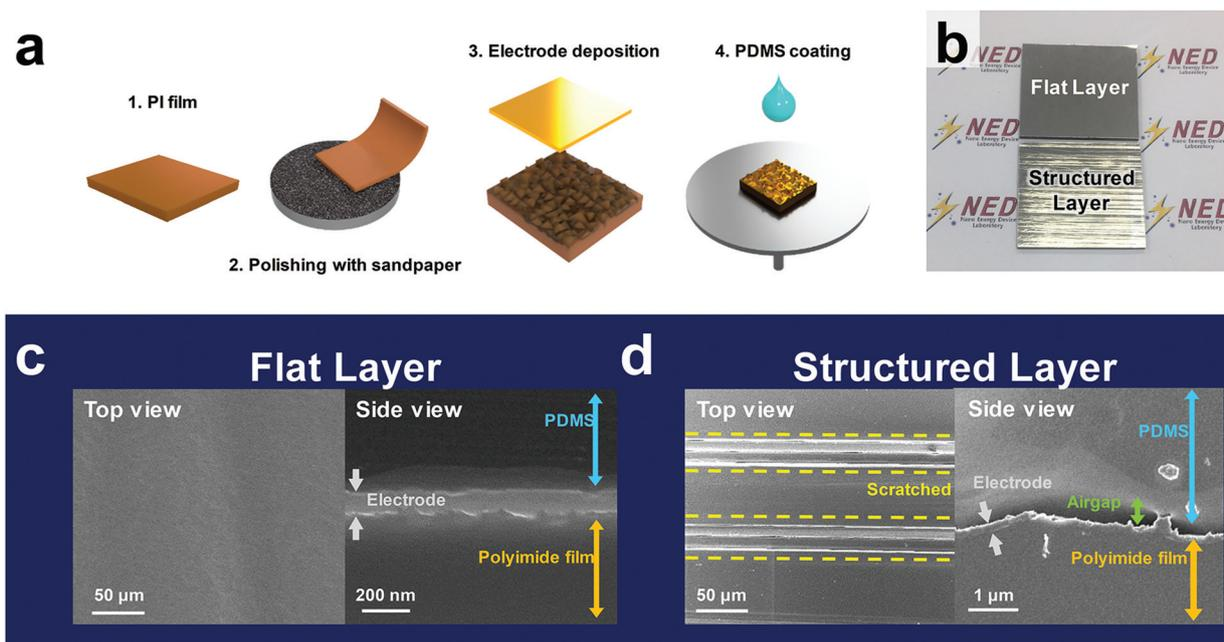
**Fig. 3** (a) Illustrated schematics of the fabrication process for the structured layer by using chemical mechanical polishing. (b) Digital photographs of the Al-coated flat and structured layer. The SEM images of the top-view and cross-section of (c) the flat layer and (d) structured layer.
