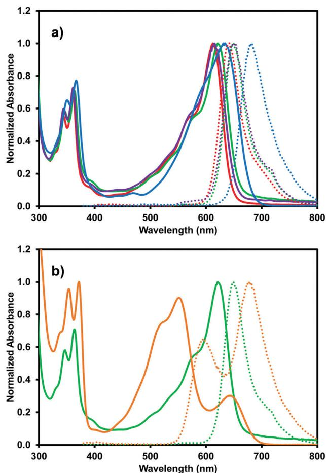
Fig. 5 (a) UV-vis absorption (solid) and emission (dot) profiles for (<sup>1</sup>PrNH)<sub>2</sub>NDI-V measured in acetone (red), DCM (green), methanol (purple), and water at pH 10 (blue); (b) absorption and emission profiles for (<sup>1</sup>PrNH)<sub>2</sub>NDI-V measured in DCM (green) and in DCM with 2.5% v/v TFA (orange). Emission was obtained with excitation at 360 nm.
