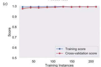
Fig. 5 The results predicting the optical emission spectrum for SiQDs, in the (a) training set, (b) testing set, and (c) the cross validation set, showing no over-fitting or under-fitting.
