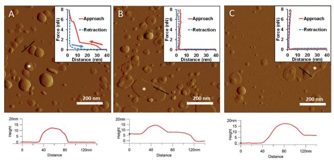
Fig. 2 Amplitude-contrast AFM image of LPS vesicles in the presence of 10 mM Ca<sup>2+</sup>; at 20 °C (A). The sample was warmed to 50 °C (B); and then cooled back to 20 °C (C). Insets: force-distance curves recorded while pressing LPS at the locations marked by the white star on each image. On the inset of A arrows indicate the direction of tip movement. Lower panels show height profiles taken along the black lines.
