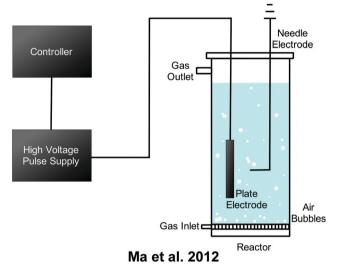
Scheme 10 Schematic representation of the SSP method carried out by Ma *et al.* and adapted from their work. <sup>121</sup> Licensed under CC BY 3.0.
