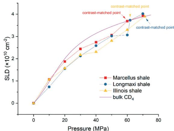
Fig. 6 Average SLD in open pores as a function of pressure for the three shale samples.
