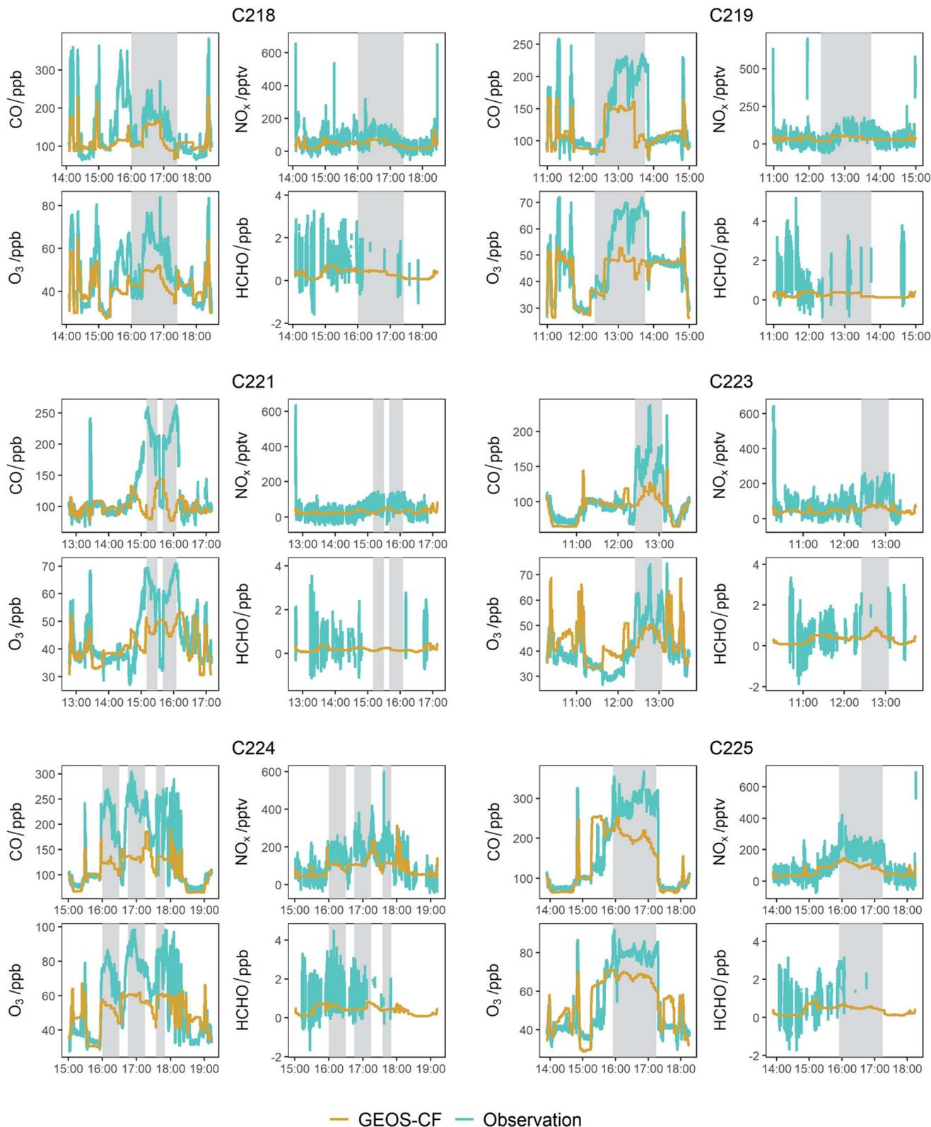
Fig. 8 Time series of measured and modelled (GEOS-CF) O<sub>3</sub>, CO, NO<sub>x</sub> and HCHO.
