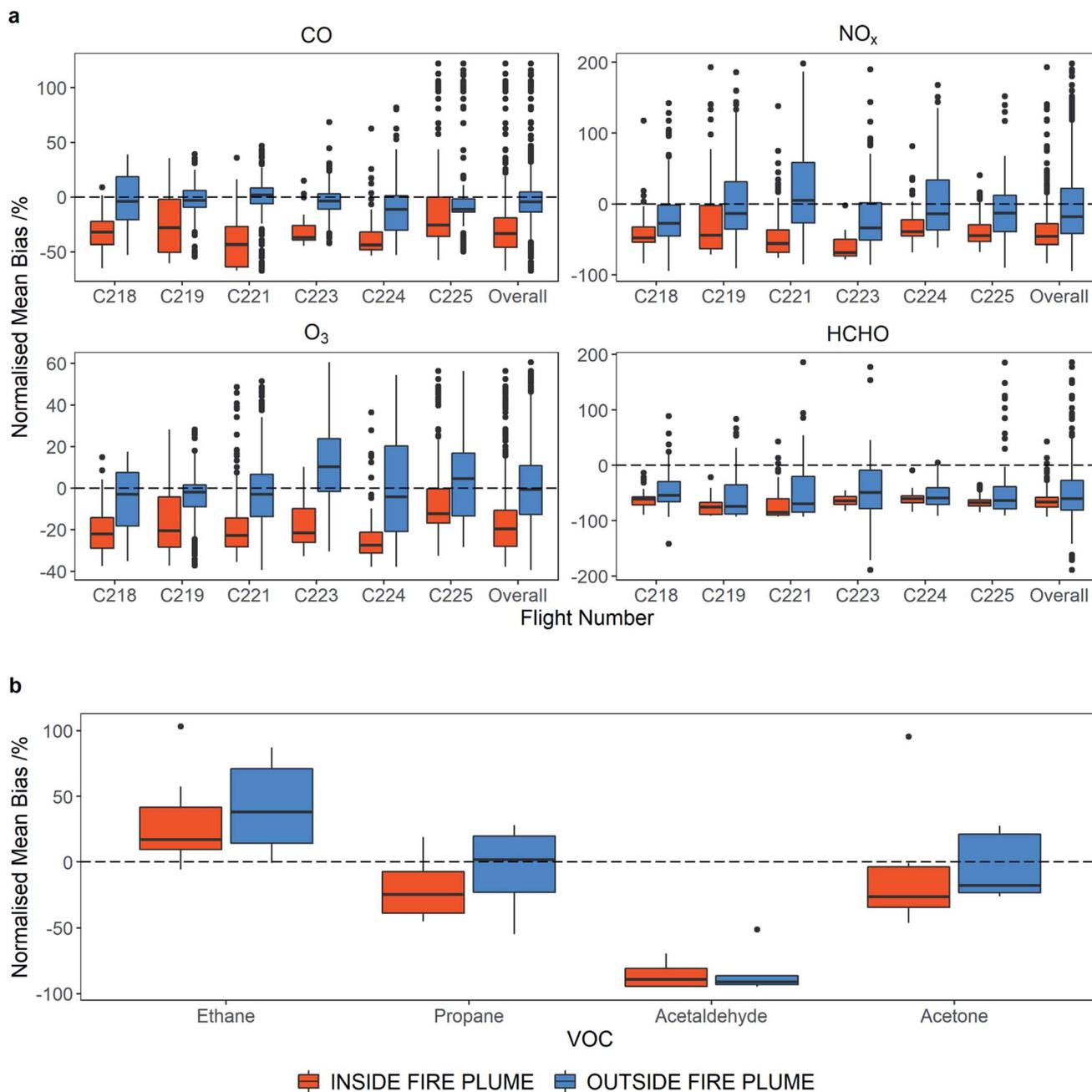
**Fig. 9** Box and whisker plots to show normalised mean bias (NMB) of the model (GEOS-CF) in and out of fire plumes for (a) CO, NO<sub>x</sub>, O<sub>3</sub> and HCHO by flight (b) VOCs for all flights. The bold horizontal lines show the median NMB, the edge of the boxes show the lower and upper quartiles, the vertical lines show the minimum and maximum values no more than 1.5 times the interquartile range and NMB values greater than these are represented by black dots.
