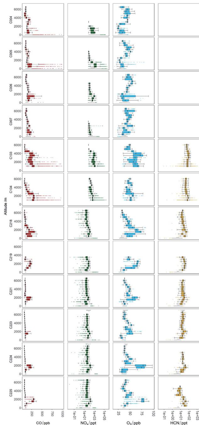
Fig. 4 Altitude binned box/whisker plots of  $\text{NO}_x$ , HCN,  $\text{O}_3$ , and CO for each flight.  $\text{NO}_x$  concentrations higher than 1000 ppt are not included in these plots so profile details are clearer at high altitude.
