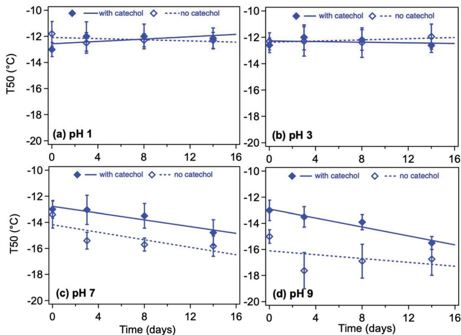
Fig. 37 Ice nucleation efficiency as gauged by  $T_{50}$  values as functions of time and starting pH of reaction and control AZTD slurries. Error bars in  $T_{50}$  represent propagated  $\pm 2\sigma$ . The figure and the caption were reproduced from ref. 206 with permission from the American Chemical Society, © 2020.
