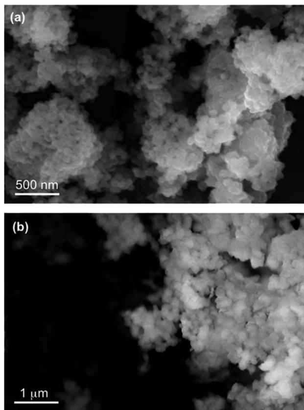
Fig. 7 SEM images of (a) polycatechol and (b) polyguaiacol collected on copper grids after a 90 min dark reaction of catechol with  $\text{FeCl}_3$  at pH 3 in a 1 : 2 molar ratio. Reproduced from ref. 70 with permission from the American Chemical Society © 2015.
