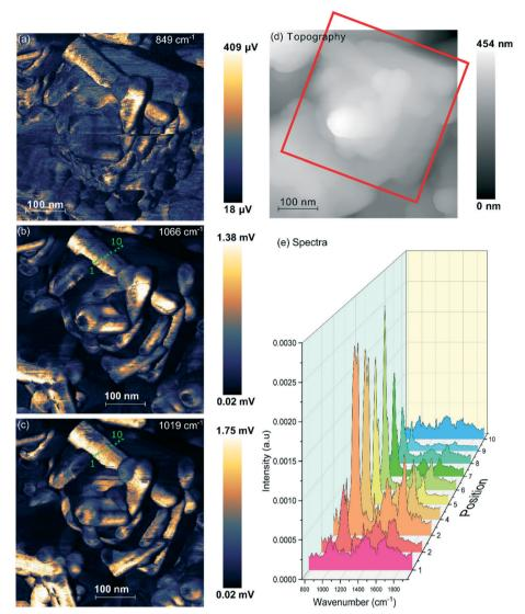
Fig. 6 PiFM images and spectra of cerium phosphate nanorods synthesised at a phosphate concentration of  $4.4 \times 10^{-3}$  M and a temperature of 170 °C. PiFM intensity maps at: (a) 849 cm<sup>-1</sup>; (b) 1066 cm<sup>-1</sup>; and (c) 1019 cm<sup>-1</sup>; (d) topography, red square indicates the outline of a CeO<sub>2</sub> cube; (e) waterfall plot of PiFM spectra across the surface (points 1-10).
