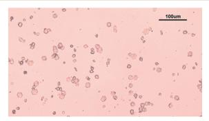
2 Rhombohedral insulin crystals obtained from crystallisation without amino acids. The conditions for the batch crystallisation matched the conditions in the sample for solubility determination and are the following: 0.48 M citric acid buffer, 0.7 mM zinc-sulphate and arginine, glycine or leucine concentration between 0.01 M and 0.1 M or without amino acids as shown here.
