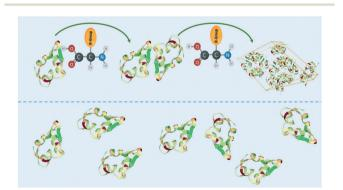
Fig. 1 Schematic showing amino acid enhancing the interaction between protein molecules (e.g. insulin) in the soft-templating concept resulting in an enhancement of nucleation and crystallisation.
