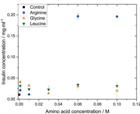
Fig. 8 Insulin solubility ( $c_e$ ) in 0.48 M citric acid buffer (pH 7) with 0.7 mM zinc sulphate at different amino acid types and concentrations.
