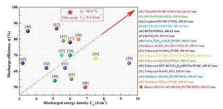
Fig. 6 Comparison of energy density and efficiency of this work (PEI-10 vol% BaTiO<sub>3</sub>/P(VDF-HFP) composite) and reported results.
