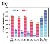
Fig. 4 (a) Weibull distribution plots and (b) characteristic breakdown strengths of the single layer and bilayer composites with different BaTiO<sub>3</sub> loading fractions.
