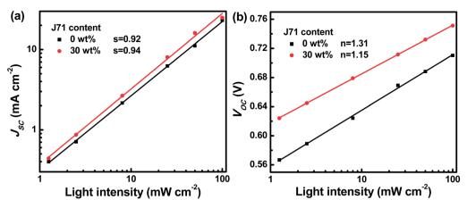
Fig. 5 (a)  $J_{SC}-I$  and (b)  $V_{OC}-I$  curves of the optimized binary and ternary OPVs.
