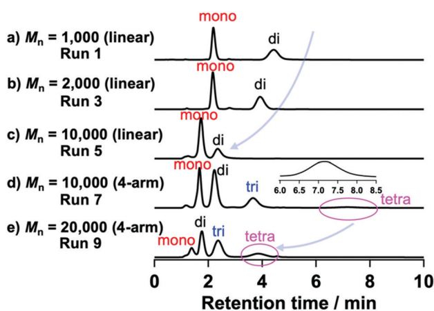
Fig. 3 HPLC profiles of modified PEGs with different molar masses and functionalities (eluent: acetonitrile/water, 45/55, v/v; flow rate: 1.0\text{ mL min}^{-1} on a C18 column at 30\text{ }^\circ\text{C} using a UV detector).
