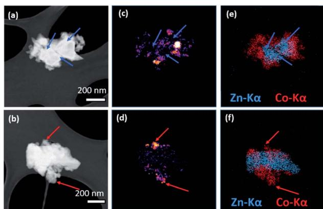
Fig. 4 Scanning transmission electron microscopy. MOF CGC particles in a  $(\text{ZIF-67})_{0.5}(\text{ZIF-62})_{0.5}$  sample. (a and b) ADF images showing particle morphology, (c and d) crystallinity maps showing the number of Bragg peaks as a function of probe position in SED data. (e and f) compositional maps of Zn and Co metal centres from STEM-EDS mapping. Arrows used to indicate correlation between the presence/absence of diffraction with that of Co/Zn.
