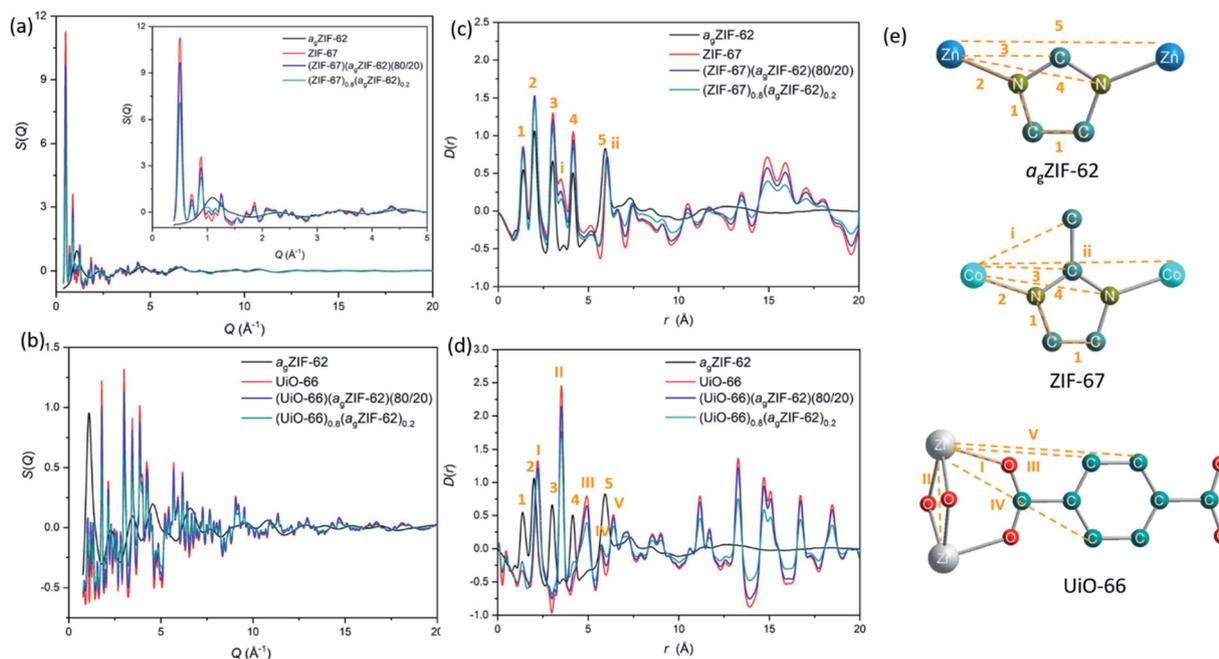
**Fig. 2** X-ray total scattering. (a and b) structure factors,  $S(Q)$ , of  $\text{a}_g\text{ZIF-62}$ , ZIF-67, UiO-66 physical mixtures and CGCs. (c and d) Corresponding pair distribution functions,  $D(r)$ . (e) Scheme of peak assignment of PDF patterns. Zn, blue; C, dark green; N dark yellow; Co, light blue; Zr, grey; O, red; H, omitted for clarity.
