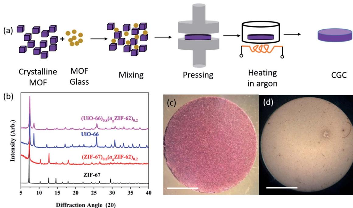
**Fig. 1** Fabrication of bulk monolithic CGCs. (a) Schematic diagram of fabrication procedure. (b) X-ray diffraction patterns of as synthesized ZIF-67 and UiO-66, alongside patterns from the CGCs. Data normalized for each sample using the intensity of the most intense peak. Optical images of (c)  $(\text{ZIF-67})_{0.8}(\text{a}_g\text{ZIF-62})_{0.2}$  and (d)  $(\text{UiO-66})_{0.8}(\text{a}_g\text{ZIF-62})_{0.2}$ , scale bar of 5 mm.
