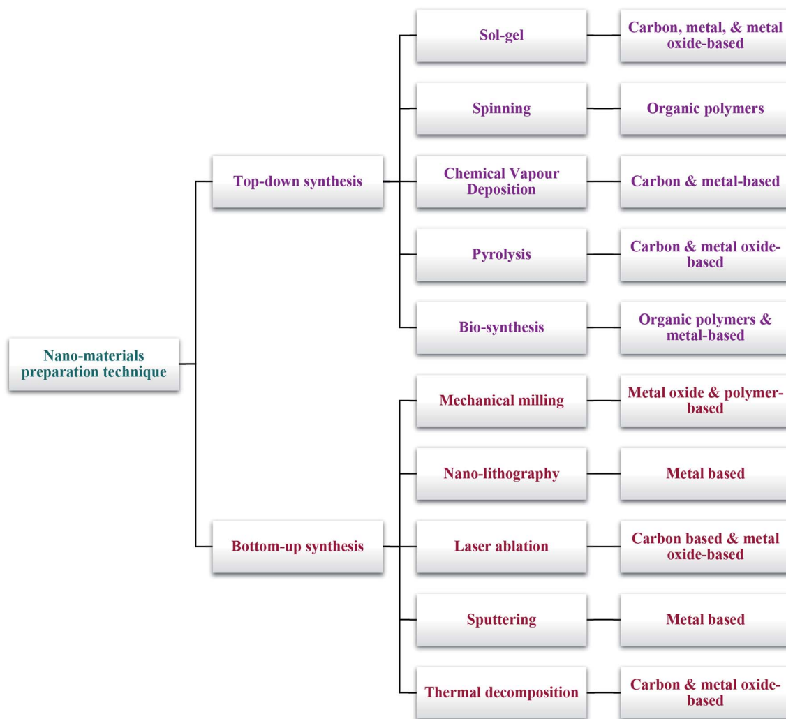
Scheme 2 Conventional synthetic techniques for nano-materials.
