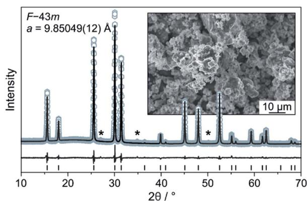
Fig. 1 Rietveld analysis of the XRD pattern for the  $Li_6PS_5Cl$  solid electrolyte. Asterisks denote impurities. The inset is a low-magnification SEM image of the as-prepared solid electrolyte powder.
