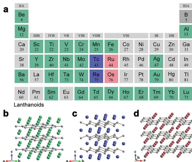
**Fig. 5** (a) Elements constructing metal diborides. Crystal structures of (b)  $AlB_2$ -type diboride; (c)  $ReB_2$ -type diboride; (d)  $RuB_2$ -type diboride. Boron is in grey, and metals used for constructing the  $AlB_2$ -type,  $ReB_2$ -type and  $RuB_2$ -type diborides are in green, blue and pink, respectively. Reproduced with permission from ref. 38. Copyright 2019 Wiley-VCH.
