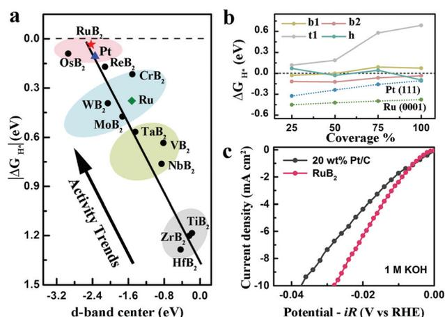
**Fig. 13** (a) Fitted linear relationship between the adsorption free energy of atomic hydrogen ( $\Delta G_{\text{H}^+}$ ) and the d-band center of  $\text{MB}_2$ , Pt and Ru. (b)  $\Delta G_{\text{H}^+}$  on the  $\text{RuB}_2(001)$ ,  $\text{Ru}(0001)$  and  $\text{Pt}(111)$  surface as a function of hydrogen coverage. (c) LSV curves for  $\text{RuB}_2$  and 20 wt% Pt/C in 1.0 M KOH solution. Reproduced with permission from ref. 38. Copyright 2019 Wiley-VCH.
