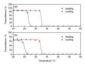
Fig. 5 Temperature dependence of transmittance at 600 nm for (a) poly(NIPAm) and (b) poly(NIPAm-g-Ala) aqueous solutions (1 wt%) in the heating (red) and cooling (blue) scan at a rate of 1 °C min<sup>-1</sup>.
