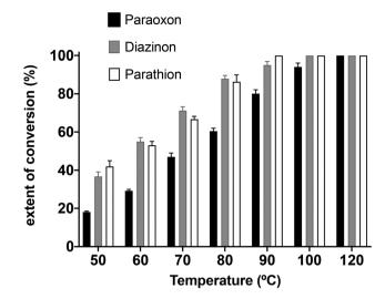
Fig. 2 Influence of MW heating on the degradation of parathion (5) (white), diazinon (4) (grey) and paraoxon (3) (black) with piperidine as the nucleophile at 50-120 °C for 30 minutes. Each experiment was performed in triplicate.
