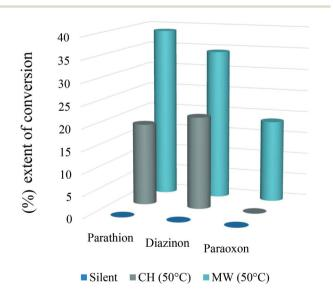
Fig. 3 Comparison of the extent of conversion (%) of pesticides after 30 minutes of reaction with piperidine as the nucleophile under MW heating (50 °C, light green blue columns), conventional heating (50 °C, dark green columns) and silent conditions (no heating, blue columns). Each experiment was performed in triplicate.
