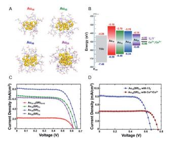
Fig. 14 (A) Geometrical structures of  $Au_x(SG)_y$  NCs (x=10,15,18 and 25). (B) Energy diagrams of the  $Au_x(SG)_y$  NCs sensitized solar cells. J-V characteristics of (C)  $Au_x(SG)_y$  NCs sensitized solar cells (x=10,15,18 and 25) with  $I^-/I^{3-}$  redox pair and (D)  $Au_{18}(SG)_{14}$  NCs sensitized solar cells with  $I^-/I^{3-}$  or  $Co^{2+}/Co^{3+}$  redox pair. Panels (a)–(d) are reproduced with permission from ref. 76. Copyright 2016 American Chemical Society.
