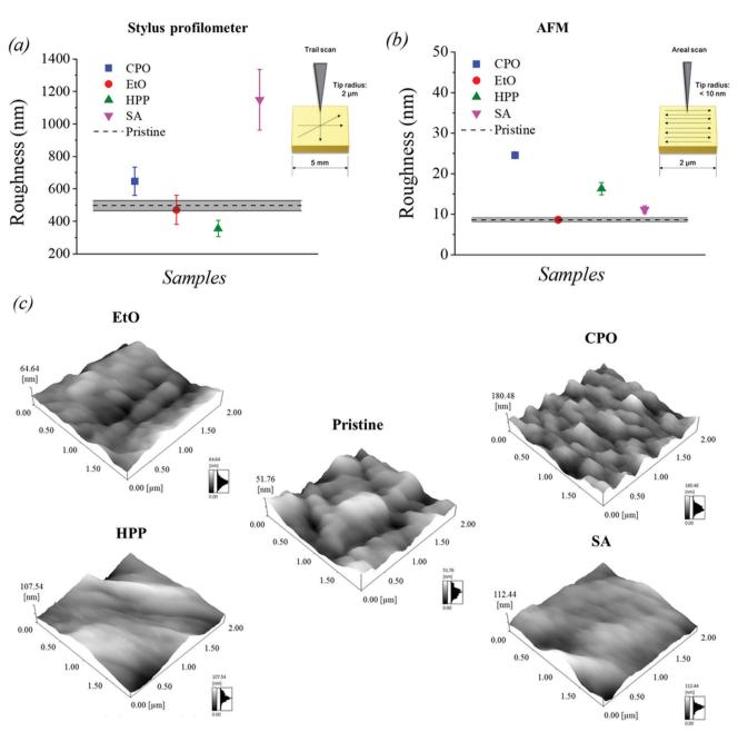
Fig. 1 Roughness (Ra) obtained by stylus profilometry (a) and AFM (b). Shaded regions represent standard deviation for pristine condition, with a continuous line. 3D profiles obtained by AFM are also displayed (c).
