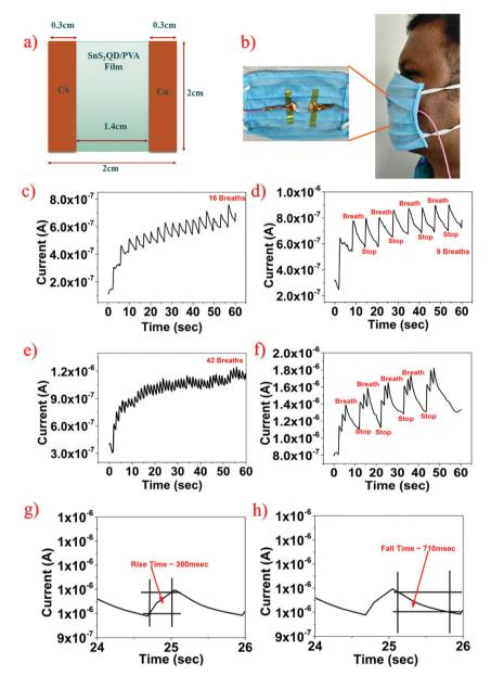
Fig. 6 (a) Schematic of a breath sensor. (b) Integration of the sensor in the breath mask. (c) Continuous-time response of  $SnS_2$  QD/PVA under normal breath. (d and e) Slow and fast breath patterns over a period of 60 seconds. (f) Three breath iterative breathing patterns for five cycles. (g and h) The rise time and fall time of the fabricated sensor were  $\sim 300$  ms and  $\sim 710$  ms.
