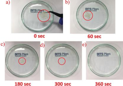
Fig. 8 Images of different stages of dissolution of SnS<sub>2</sub> QDs with the PVA substrate in DI water: (a) 0 s, (b) 60 s, (c) 180 s, (d) 300 s and (e) 360 s.
