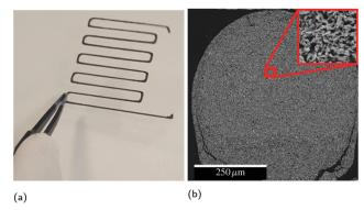
(a) Free-standing printed conductive structure after reaction of printed ball milled powders. (b) Cross-sectional electron micrograph of reacted conductive line, demonstrating bi-continuous microstructure.
