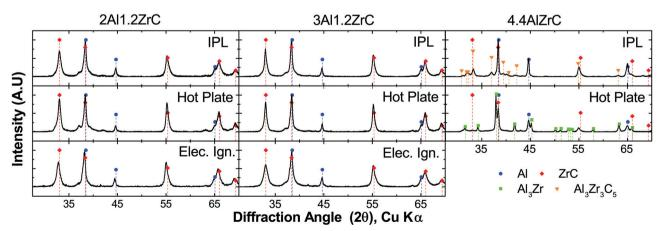
Fig. 3 Comparison of phases formed in 2Al, 3Al and 4.4Al thin films after reactions ignited by IPL, hot plate, and electric spark. Arranged in order of decreasing uniformity of energy delivery to the sample during ignition, demonstrating that for compositions too rich in Al, only very uniform ignition can produce the desired product phases. Note that 4.4Al foils would not propagate from an electric spark.
