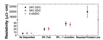
4-Point probe measured resistivities of RAIL thin films before and after reaction under IPL along with an SHS reacted printed line of PVD particles. Error bars show standard deviation of the measurement, and do not include estimates of error for assumed thickness or contact resistance
