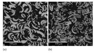
Cross-sectional electron micrographs of syringe-printed PVD particles (a) as printed and (b) after reaction. The black background is mounting epoxy.
