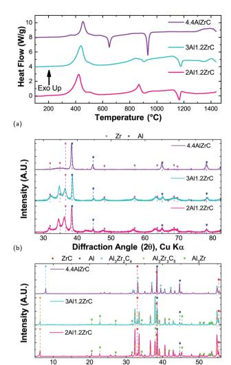
Fig. 6 (a) Heat flow *versus* temperature curves for multilayer foils heated to  $1450~^{\circ}\text{C}$  in a TA Instruments Q600. Baseline fit to a second run on the post-reacted sample. (b) X-ray diffraction patterns of multilayer foils in their as-deposited state. (c) X-ray diffraction patterns of multilayer foils after heating to  $1450~^{\circ}\text{C}$ .
