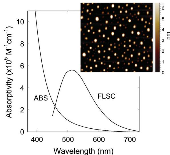
Fig. 2 Optical absorption (ABS) and fluorescence (FLSC) spectra of PEI<sub>600</sub>-CDots in aqueous solution. Inset: Representative AFM images for the CDots.
