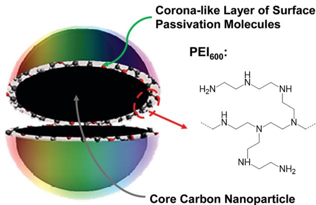
Fig. 1 A cartoon illustration on the structure in CDots in general and PEI<sub>600</sub>-CDots specifically.
