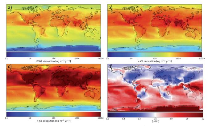
Fig. 2 Spatial distribution of modeled 2013–2015 annual average (a) PFOA deposition (ng per m<sup>2</sup> per year), (b) deposition of all longer-chain PFCAs (ng per m<sup>2</sup> per year), (c) deposition of all shorter-chain PFCAs, and (d) precursor-produced long-chain (>C7) to short-chain deposition ratio.
