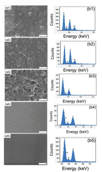
Fig. 4 Top-view SEM images of (a1) Fe-ADA, (a2) Fe-ADA-Fe-TPA, (a3) Li-ADA, (a4) Ca-ADA, and (a5) Ca-ADA@Ca-TPA; the scale bar is 200 nm in each image. The corresponding EDX pattern is given in section b.
