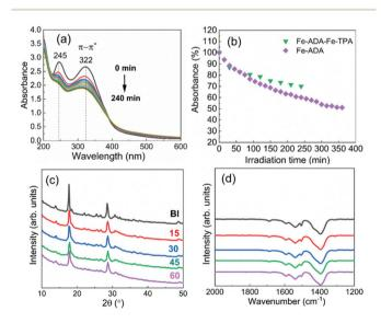
Fig. 8 (a) UV-vis spectra for Fe-ADA-Fe-TPA film after UV irradiation for different time periods in intervals of 30 min; (b) photoisomerization rate comparison; (c) GIXRD patterns, and (d) FTIR spectra for Fe-ADA-Fe-TPA film after UV irradiation for different time periods in intervals of 15 min
