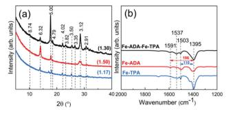
Fig. 7 (a) GIXRD patterns and (b) FTIR spectra of Fe-TPA, Fe-ADA, and Fe-ADA-Fe-TPA; numbers in parentheses in (a) are density values and the peak positions are indicated with the d-values (in A).
