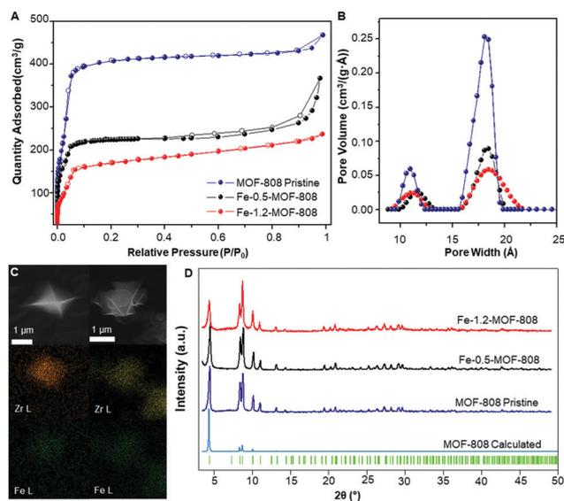
**Fig. 1** (A)  $\text{N}_2$  adsorption/desorption isotherms at 77 K showing the decrease in surface area upon iron incorporation. (B) Pore size distribution (PSD) data for pristine and Fe-SIM MOF-808 materials. (C) Mapping of Zr (yellow) and Fe (green) for Fe-0.5-MOF-808 (right) and Fe-1.2-MOF-808 (left). (D) PXRD data of the synthesized materials and their comparison with the calculated data for MOF-808,<sup>19</sup> including Bragg positions.
