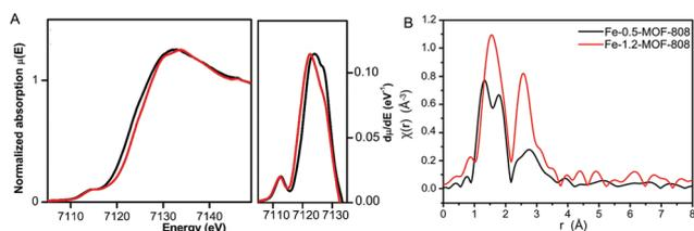
Fig. 3 (A) Fe K-edge XANES data of Fe-MOF-808 materials (left) and first derivate analysis (right) showing the rising-edge shift between both materials. (B) The  $k^3$ -weighted  $\chi(r)$  Fe K-edge EXAFS spectra of Fe-0.5- and Fe-1.2-MOF-808 systems.
