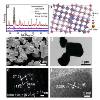
Fig. 1 (a) XRD pattern, (b) crystal structure, (c) FESEM image, (d) TEM image, (e) SAED pattern, and (f) HRTEM image of HfNb<sub>24</sub>O<sub>62</sub>. R<sub>wp</sub>: weighted profile residual.
