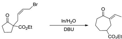
Scheme 7 In-mediated carbocyclic ring expansion in water.
