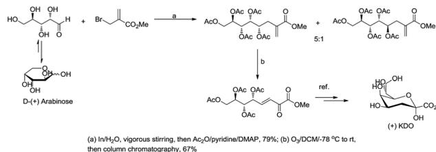
(a) InH<sub>2</sub>O, vigorous stirring, then Ac<sub>2</sub>O/pyridine/DMAP, 79%; (b) O<sub>3</sub>/DCM/−78 °C to rt, then column chromatography, 67%
