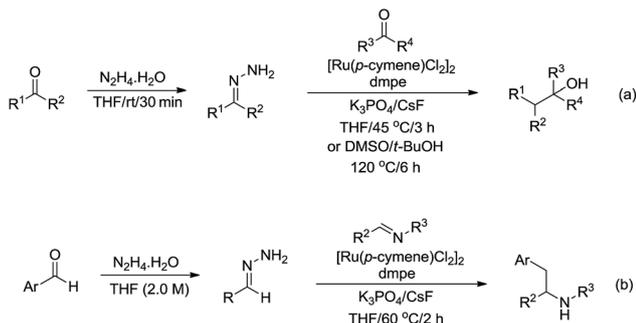
Scheme 48 Ru-catalysed nucleophilic addition of carbonyl and aryl imine compounds via hydrazone intermediate using aldehydes as carbanion equivalents.
