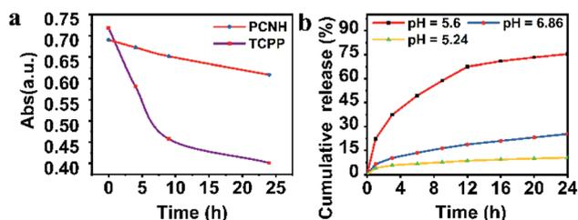
Fig. 4 Photostabilities of PCNH and TCPP when exposed to natural light for 24 h (a). Cumulative release of TCPP from PCNH in different pH solutions (b); the concentration of PCNH is 1 mg mL<sup>-1</sup>.
