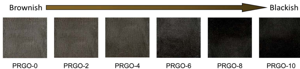
Fig. 2 Colour appearance of PRGOs deposited on the surface of a 100-mesh stainless-steel wire mesh.
