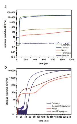
Fig. 2 Representative photorheology of monomer-derived resins over 1200 s (a) and comparing monomer and prepolymer nerol and geraniol over 3.5 h (b) as determined by network storage moduli.
