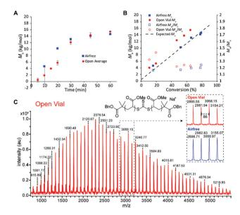
Fig. 4 Comparing the open vial polymerization to the analogous airfree reaction: (A) Mn increase over time (open vial polymerization average of three runs). (B)  $M_n$  versus conversion to show linear increase (note only one open vial trial shown, conversions for the open vial are estimated due to monomer evaporation). (C) MALDI-TOF analysis of low molecular weight samples to verify the TTC moiety and end groups remain intact for both cases.
