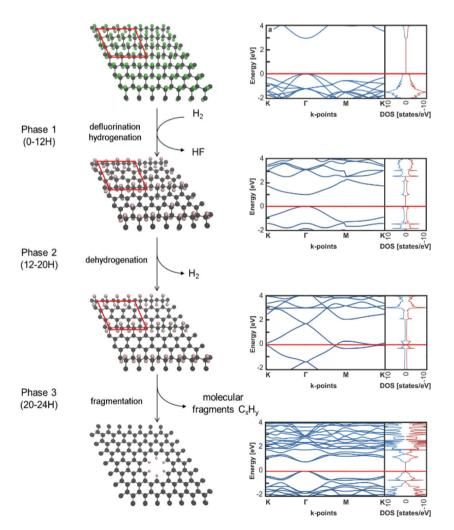
Scheme 1 Proposed mechanism of defluorination of the fluorographene sample under a reducing hydrogen atmosphere. The Fermi level in the band structure and DOS (states per eV per computational cell) is set to zero.
