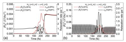
Fig. 6 Variation of the square of velocity (solid lines) in the  $Z(|\dot{R}_z|^2, \text{ panel (a)})$  and  $r(|\dot{R}_r|^2, \text{ panel (b)})$  directions along with the corresponding friction coefficients (dotted lines), as a function of time for a representative trajectory for  $H_2$  (v = 3, j = 2) to  $H_2$  (v = 2, j = 2) scattering on Ag(111), at a translational energy of 0.1 eV.
