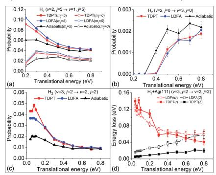
Fig. 5 (a) Vibrational state-to-state deexcitation probabilities from  $H_2$  (v=2, j=5) to  $H_2$  (v=1, j=5) for rotationally excited initial conditions as predicted with MD, MDEF(LDFA), and MDEF(TDPT). (b) Vibrational excitation probabilities upon scattering. (c) Vibrational deexcitation probability from  $H_2$  (v=3, j=2) to  $H_2$  (v=2, j=2). (d) Energy loss during vibrational deexcitation from  $H_2$  (v=3, j=2) to  $H_2$  (v=2, j=2).
