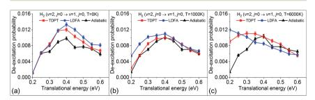
Fig. 7 Vibrational deexcitation probabilities from  $H_2$  (v=2, j=0) to  $H_2$  (v=1, j=0) simulated by MD, MDEF(LDFA), and MDEF(TDPT), with electronic temperatures of 0 K (a), 1000 K (b), and 6000 K (c).
