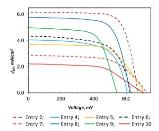
Fig. 1 Current density-voltage characteristics of masked DSSCs in the presence of D1 as the dye and various electrolytes.
