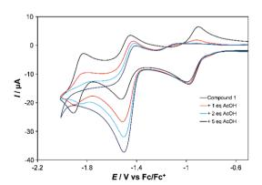
Fig. 3 CV showing effect of adding 1, 2 and 5 equivalents of AcOH to the first two reduction waves of 1 in MeCN. Conditions as described under Table 1.
