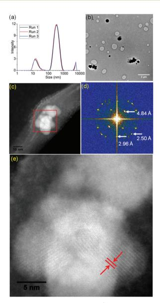
**Fig. 3** (a) DLS spectra of **FeMs** (1 mg mL $^{-1}$ , H $_2$ O) from three independent experiments (assigned as runs 1, 2, 3). (b) TEM image of the Fe-nanoclusters. (c) STEM image of Fe-nanoclusters. (d) FFT and the measured *d*-spacings of multiple planes. (e) Lattice within the Fe-rich nanoparticle.
