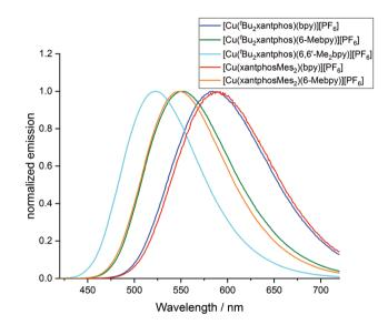
Fig. 12 Normalized solid-state emission spectra of  $[Cu(P^P)(N^N)][PF_6]$  complexes ( $\lambda_{exc}$  = 365 nm).
