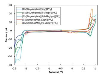
Fig. 9 Cyclic voltamogramms of [Cu(P^P)(N^N)][PF<sub>6</sub>] compounds in  $CH_2Cl_2$  at a scan rate of 100 mV s<sup>-1</sup> referenced to internal Fc/Fc<sup>+</sup> = 0 V.
