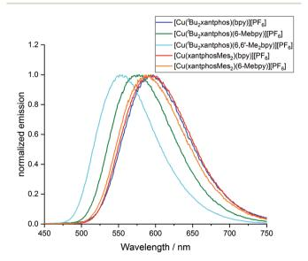
Fig. 13 Normalized emission spectra of [Cu(P^P)(N^N)][PF<sub>6</sub>] complexes in Me-THF at 77 K ( $\lambda_{exc}$  = 410 nm).
