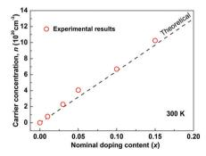
Fig. 2 Carrier concentration as a function of the nominal doping content at room temperature in  $Cu_3Sb_{1-x}Sn_xS_4$  system. The dashed line is the theoretical model where a full charge transfer is assumed (one hole carrier per dopant).
