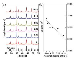
Fig. 1 (a) XRD patterns and (b) compositional variation of unit cell volume in Cu<sub>3</sub>Sb<sub>1-x</sub>Sn<sub>x</sub>S<sub>4</sub> system.
