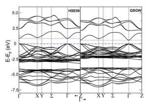
Fig. 7 Band structure for  $Cu_3SbS_4$  for spin-orbit coupling calculation with hybrid-DFT (HSE06, left panel) and QSGW (right panel). All the energies in eV referred to the Fermi energy.
