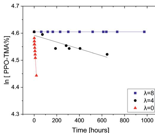
Fig. 1 Remaining PPO-TMA fractions as a function of time with hydration number  $\lambda = 0, 4$  and 8, in 0.06 M OH<sup>-</sup> DMSO-d<sub>6</sub> solutions. All tests were done at room temperature.
