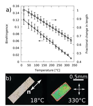
Fig. 7 (a) Fractional length change and birefringence of a sample as it is heated from 18 °C to 330 °C. For clarity, errors have been enlarged by a factor of 5. (b) Corresponding polarising microscopy images of the sample at 18 °C and 330 °C. The director, n, has been marked on the photograph of the sample at 18 °C and remained in the same orientation at 330 °C.
