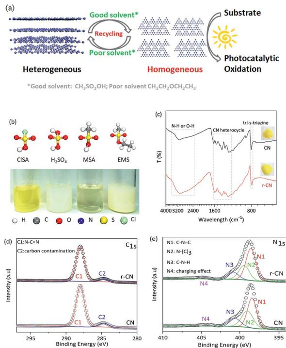
Fig. 1 (a) Bridging homo/heterogeneous photocatalysis. (b) A photo of CN in sulfonic acid group-containing solvents ( $50 \text{ mg mL}^{-1}$ ) at room temperature, and a ball-and-stick model of the solvents. Bulk CN was only completely dissolved in MSA. (c) FT-IR, (d) XPS C 1s and (e) N 1s spectra of bulk CN and that recovered from the MSA solution (r-CN). Inset: photos of CN and r-CN.
